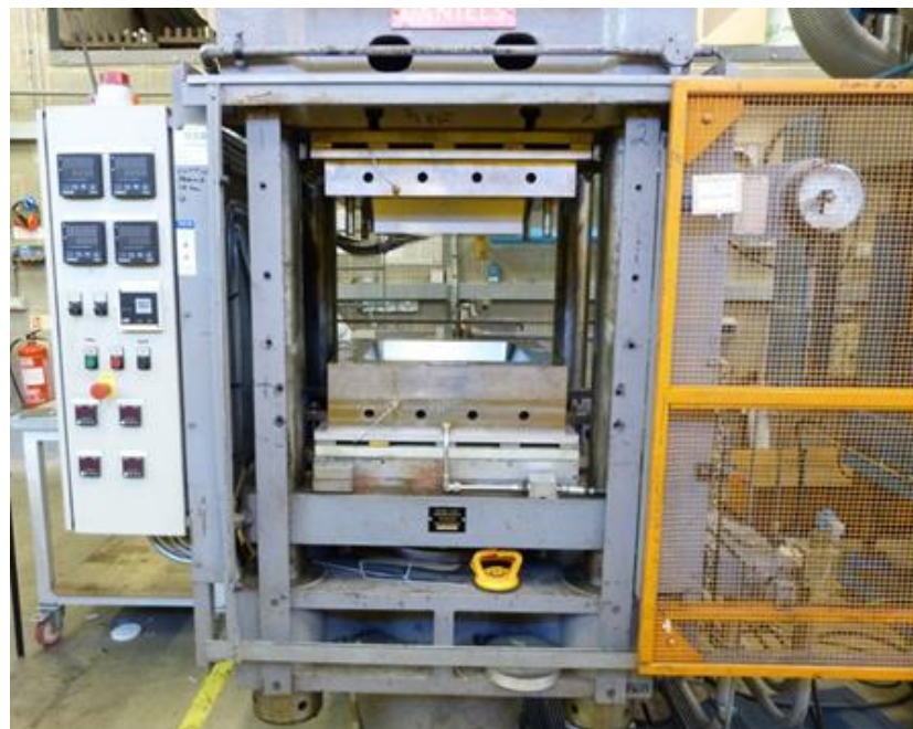
Figure 31: Daniels upstroke press with heaters and pressure transducer labelled
