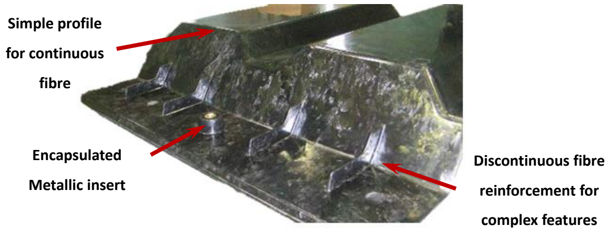
Figure 19: Mitsubishi Rayon prepreg compression moulding demonstrator component [71]
