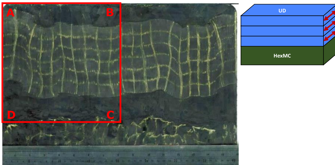
Figure 89: U3 0° H2 60% plaque with the testing region shown as a red square. Charge construction diagram (red arrows indicate UD fibre direction). A to D represent plate locations for Figure 91
