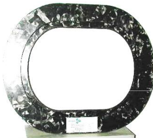
Figure 6: Boeing 787 window frame from carbon fibre sheet moulding compound [24]
