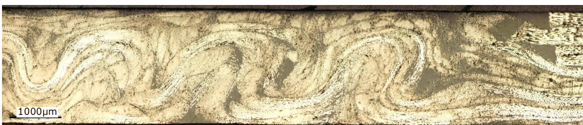
Figure 117: Micrograph of U3 0° H2 s50%, showing a rippled region.
