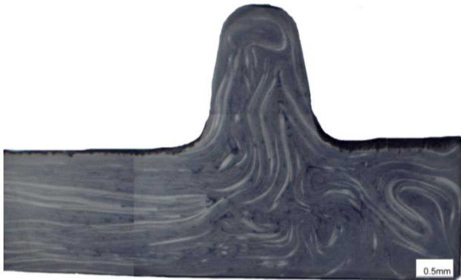
Figure 140: Micrograph of rib and plate edge on the right
