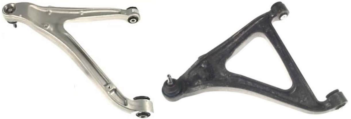
Figure 5: Replacement of aluminium with carbon fibre SMC in a front lower control arm of the Lamborghini Sesto Elemento [21]
