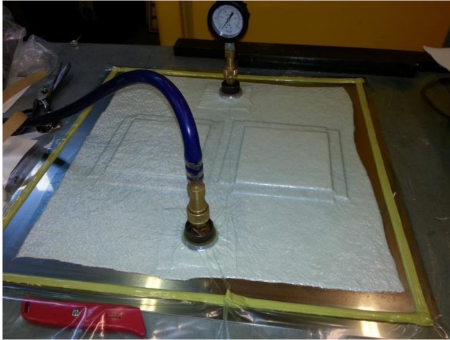
Figure 43: Bagging for out-of-autoclave with corking for staging trials
