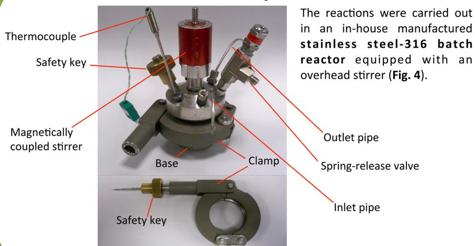
Fig. 4 – Stainless steel clamp-sealed vessel used for the polymerisations.
