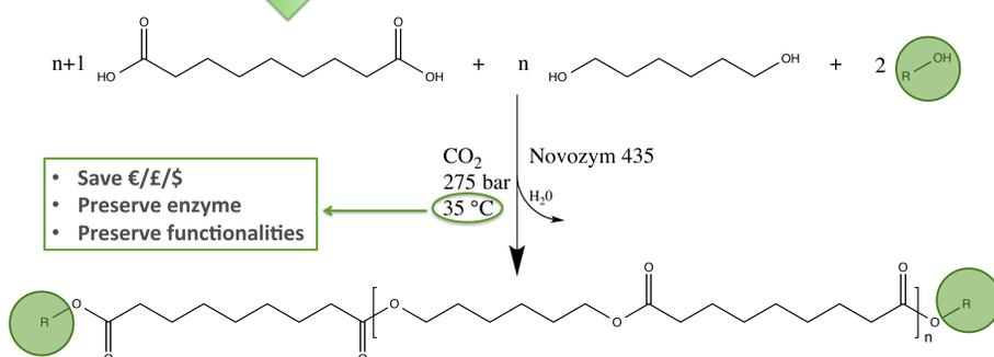
Fig. 2 – Synthesis of functional poly(hexylene azelate) (PHA) in scCO<sub>2</sub>.
