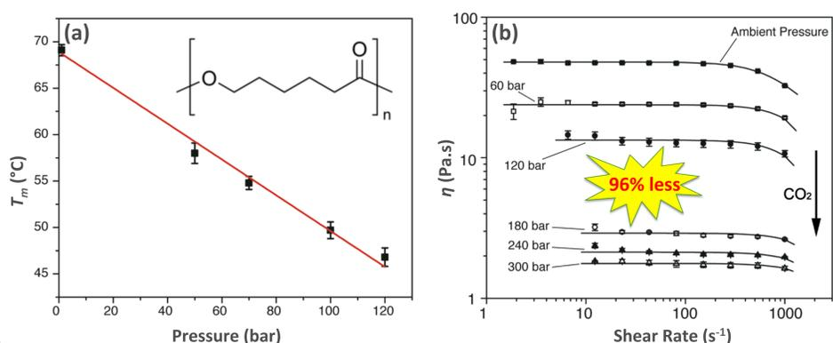
Fig. 1 – Effects of CO<sub>2</sub> on the T<sub>m</sub> (a) and viscosity (b) of PCL (M<sub>n</sub> ~10 kDa). The polymer structure is shown (inset).
