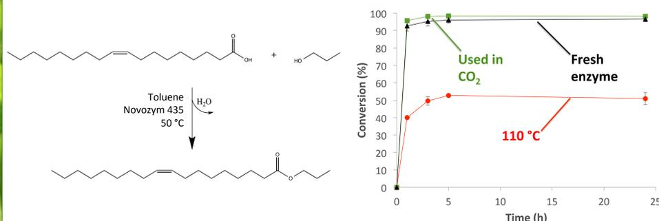
Fig. 5 – Synthesis of propyl oleate (left) and reaction conversion (through <sup>1</sup>H-NMR, right) when using new Novozym 435 and enzyme after: five CO<sub>2</sub> reactions and a reaction in the melt (110 °C)
