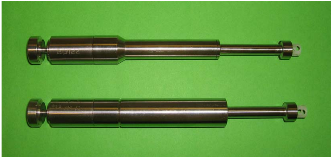
Fig. 2.2: Laboratory versions of the inverting dome device, with and without a silencer.
