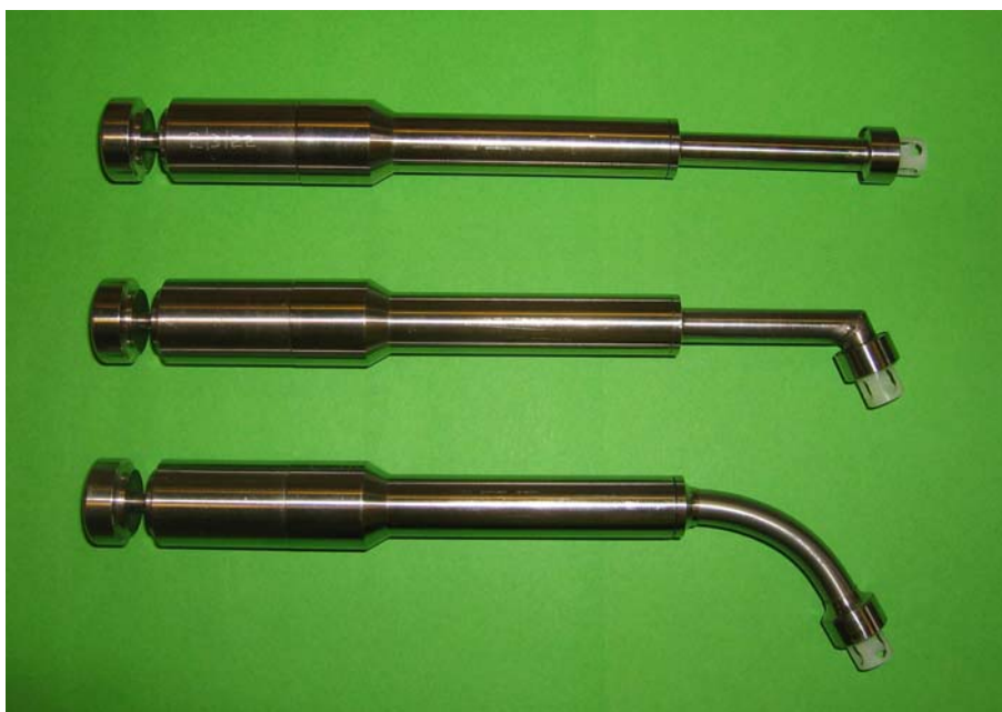
Fig. 1.2: Laboratory versions of the inverting dome devices, shown straight and with bent and kinked shock tubes. Devices similar to these were used in the 1998 clinical trial [15].
