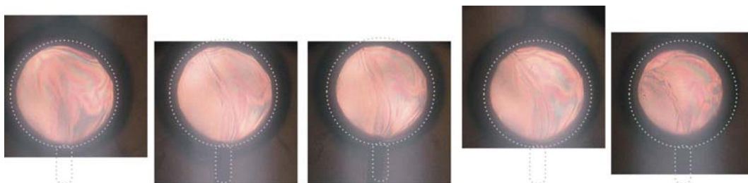
Fig. 3.12: Five injection-moulded discs viewed through polarised light. The dimensions of the disc and the position of the injection-moulding gate is shown with a dotted line.
