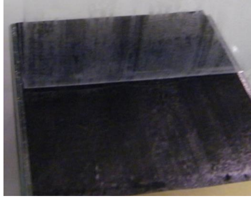
Figure 10: Longitudinal resin bands on FEP film.
