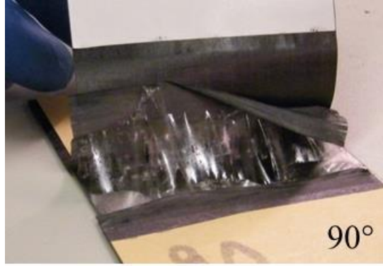
Figure 8: Effect of ply angle on measured prepreg-prepreg tack
