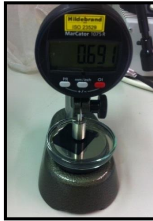
Figure 116. Measurement set up for measuring of thickness during swelling state using a Hildebrand rubber thickness gauge.
