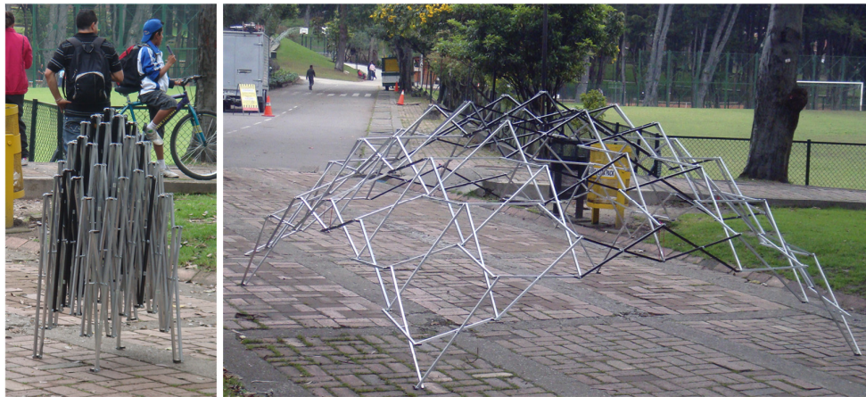
Figure 5.1 A synclastic surface using curved-translational scissors. (Gómez Lizcano, 2012).
