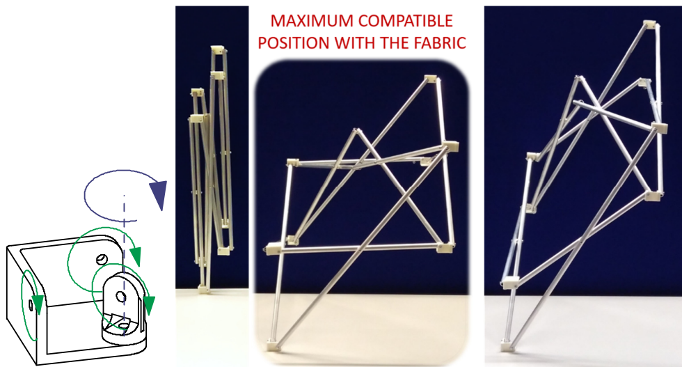
Figure 5.20 Manufactured sample of an approximated stress-free oblique rhomboidal prism with single diagonalisation and rotary joints.
