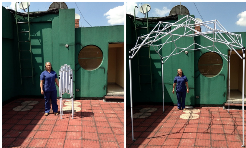
Figure 5.2 A synclastic surface using curved-translational scissors and telescopic legs. [Personal library -unpublished work, 2014].
