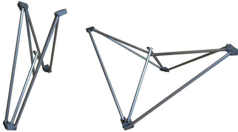
Figure 5.8 Manufactured sample of Calatrava's square-base model.
