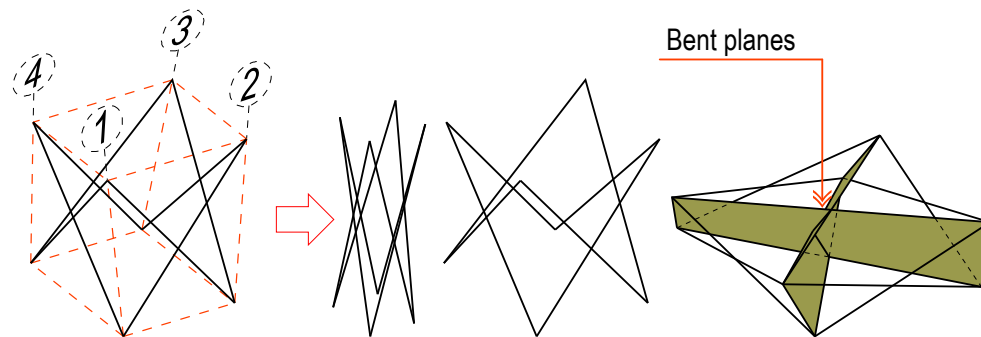
Figure 4.41 A sliced tetrahedron utilised in the prior art.
