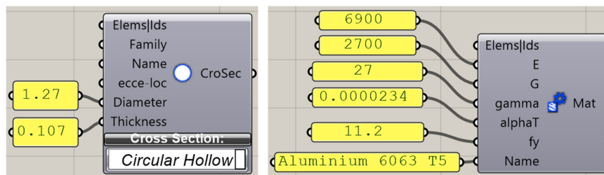
Figure 6.3 Cross-sections and material properties.
