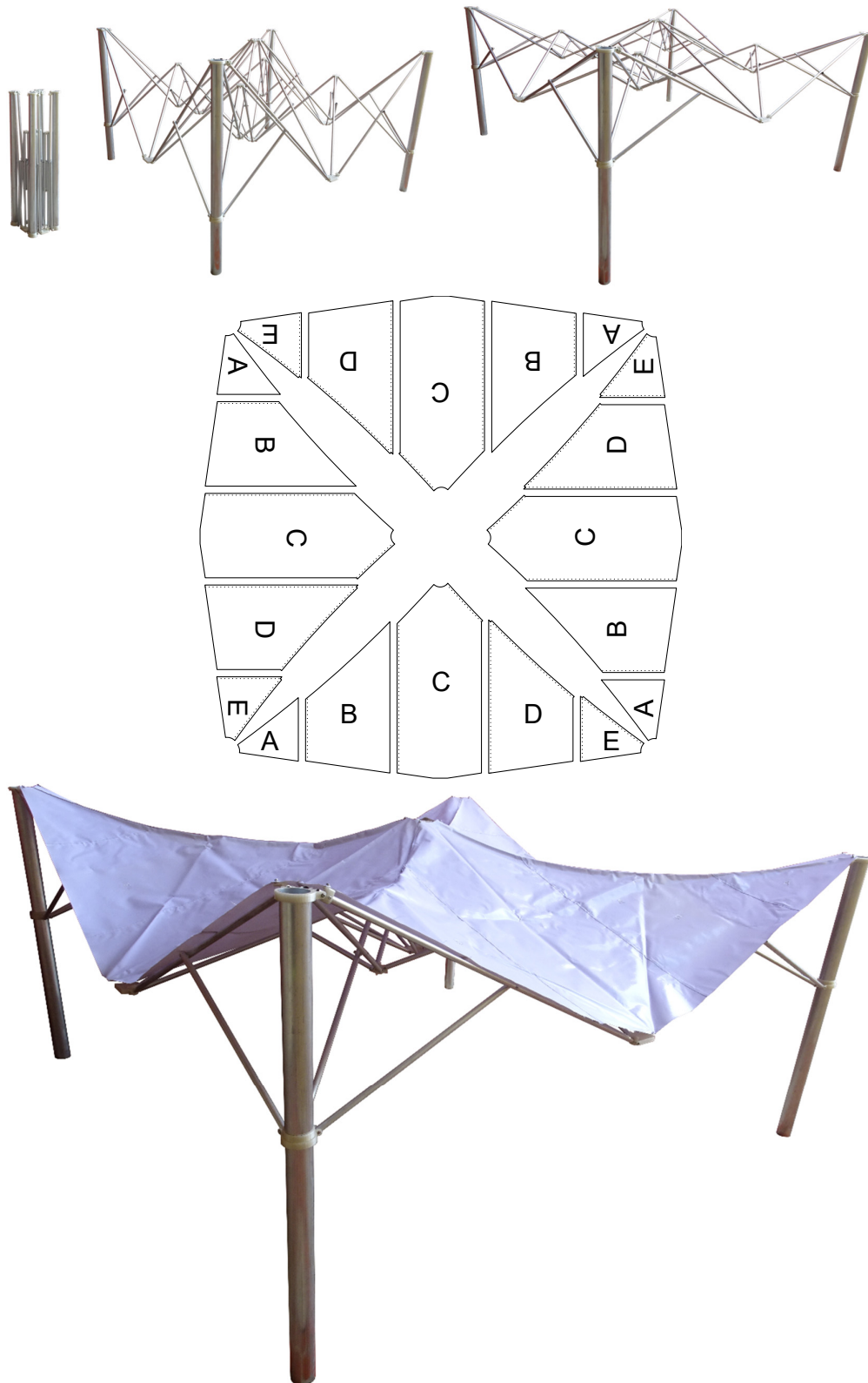
Figure 5.27 A deployable Hypar tent scale model and cutting patterns for the fabric.
