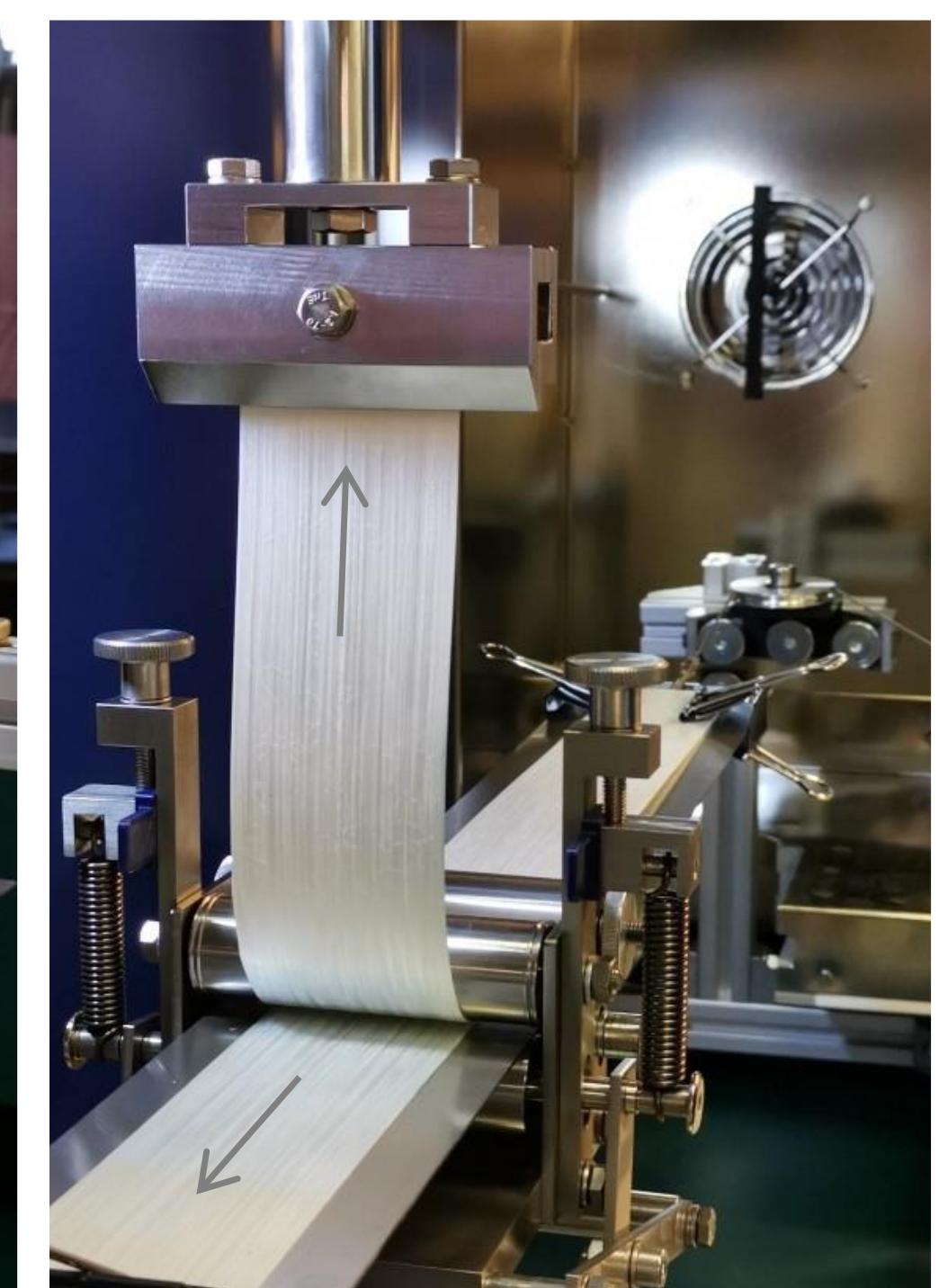
Figure 4 Peel test rig configuration with applied back tension.
