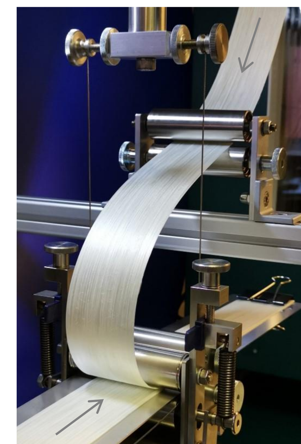
Figure 3 Consolidation test rig configuration.
