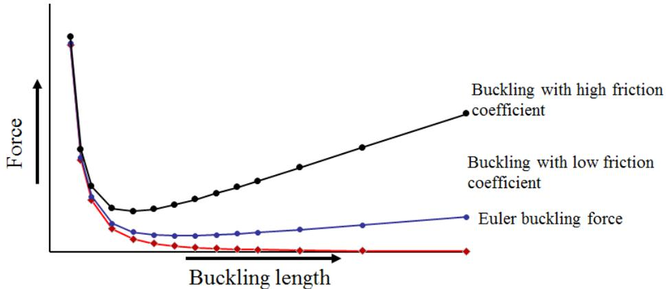
Figure 5. Effect of substrate friction on buckling of a beam
