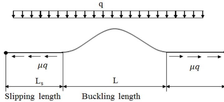
Figure 4. Buckling model
