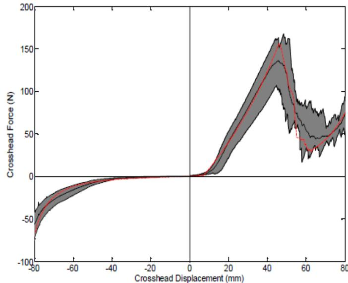
Figure 1. Shear curves for NCF [8] (black curve – average experimental response, grey shaded area – scatter of experimental results)
