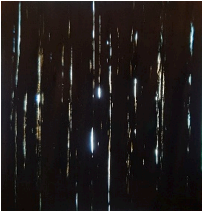
Fig. 5. Backlit image of a HT peeled PA6 tape qualitatively showing splitting and fibre waviness caused by the peeling process.
