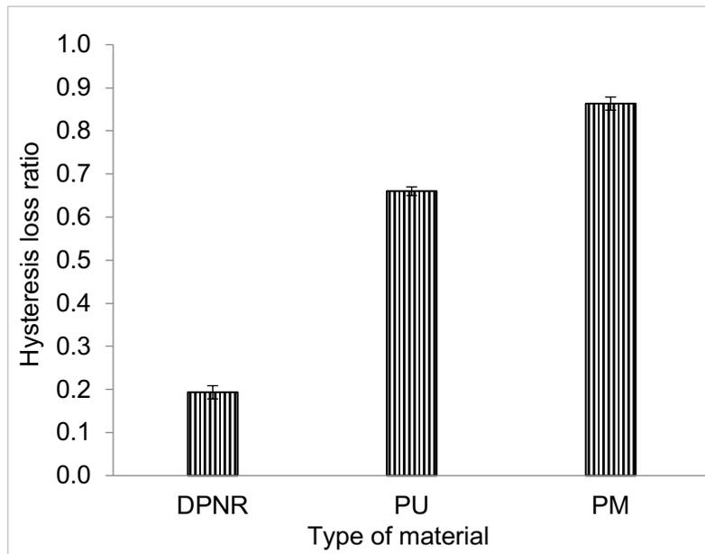
Fig. 3: Hysteresis loss ratio of DPNR latex foam, PU foam, and PM foam
