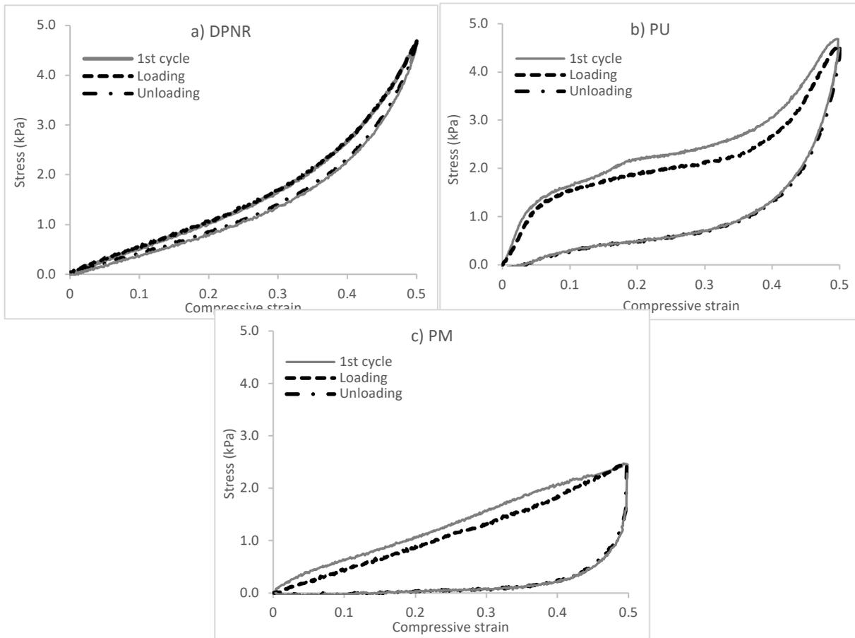
Fig. 2: Loading-unloading curve of a) DPNR latex foam, b) PU foam, and c) PM foam. The solid line represents the first cycle, the dash line represents the third cycle.
