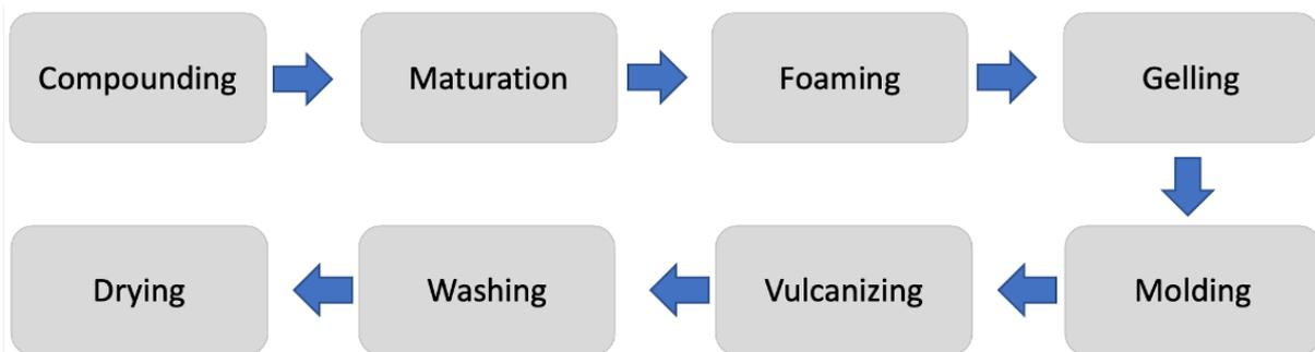
Fig. 1: The different stages involved in the production of DPNR latex foam
