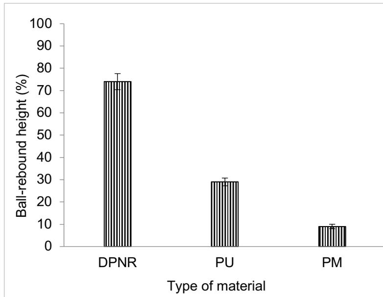
Fig.4: Percentage of rebound height of DPNR latex foam, PU foam, and PM foam
